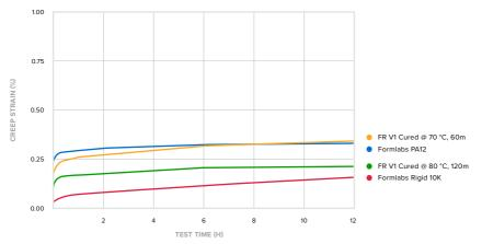
Formlabs Flame Retardant Resin parts have high creep resistance. Post-curing Flame Retardant Resin samples at 80 °C for 120 minutes shows improved creep resistance compared to post-curing at 70 °C for 60 minutes. Flame Retardant Resin samples post-cured at 80 °C and 120 minutes is slightly lower in creep resistance than Rigid 10K Resin samples. Flame Retardant Resin samples post-cured at 70 °C and 60 minutes showed similar creep behavior as Formlabs Nylon 12 SLS Powder.
