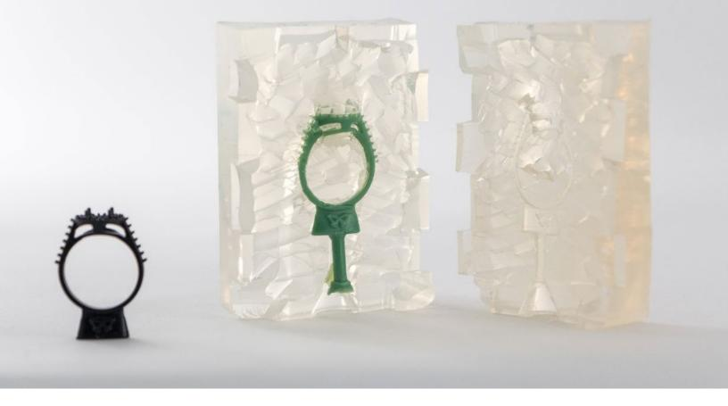
RTV silicone may be clear, which can be helpful when cutting molds with complex geometries.
