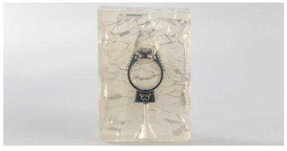
RTV molding does not require a vulcanizer and has a lower up-front investment, but ongoing material costs may be higher.
